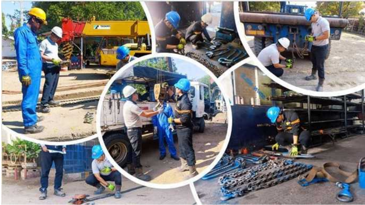
Figure 54: Lifting Gear, Hoisting & Handling Equipment NDT Inspection and Color Coding
