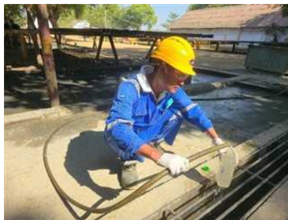
Figure 44: Water Sample Collection at Warehouse Zero Discharge Tank
