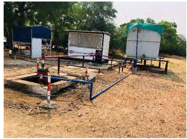
Figure 44: Produced Water Injection at Shut-in Wells
