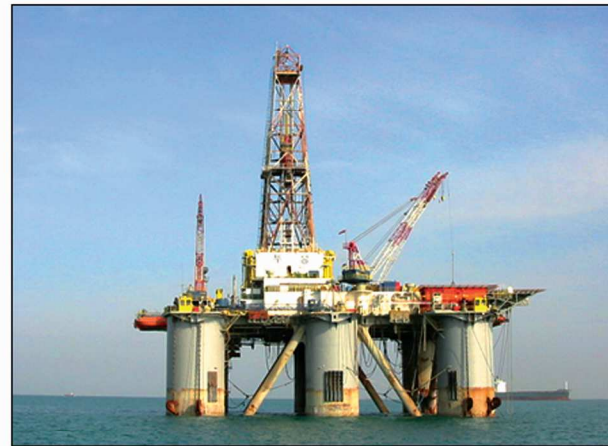
Fig. 4: KNOC's Doosung Semi-sub Drilling Rig used to drill Well Pyi Thar-1 and its Geological Sidetrack
